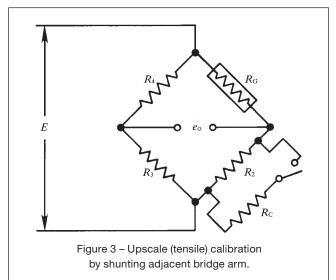
for most practical applications. The error in the simulated tensile strain, in percent, is approximately equal to the gage factor times the strain, in percent.
