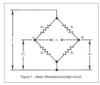
in output voltage due to decreasing any one of the arm resistances by shunting. The equation also demonstrates that the sign of the change depends on which arm is shunted. For example, decreasing  $R_1/R_2$  by shunting  $R_1$ , or increasing  $R_4/R_3$  by shunting  $R_3$  will cause a negative change in output. Correspondingly, a positive change in output is produced by shunting  $R_2$  or  $R_4$  (increasing  $R_1/R_2$  and decreasing  $R_4/R_3$ , respectively).
