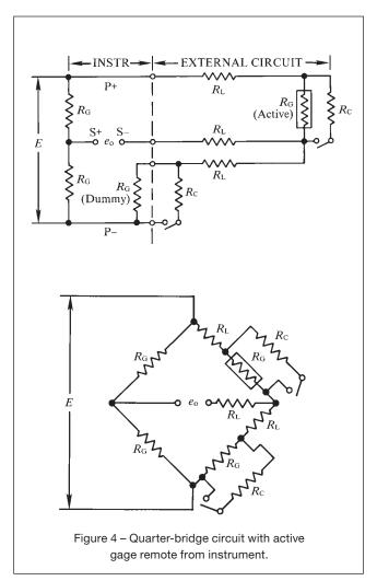
After adjusting the sensitivity of the instrument to register the calibration strain, the effect of the leadwire resistance is eliminated from all subsequent strain measurements.
